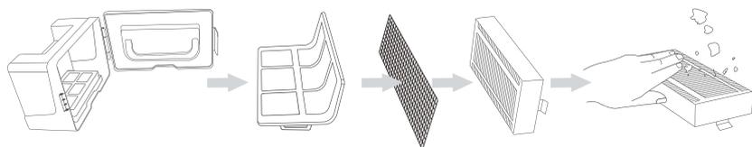
4. Wash the dust collector and the first filter element, dry the dust collector and filter elements, and keep them dry to ensure their service life
